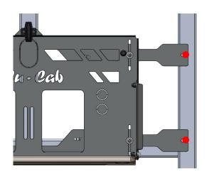
Mark the hole position for the M8 Rivnuts and using an 11mm drill bit, drill holes in the canopy camper door frame being careful to only drill though the single wall of the aluminum extrusion.
