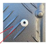
**A.** Locate the rivets that mount the bags to the inside of the rear door and drill them out from the outside of the door.
