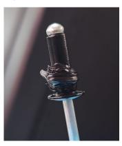
**B.** Place a small piece of sealant (preferably SikaFlex) on the black rivets supplied in the kit to plug up the holes made from drilling out the rivets.
