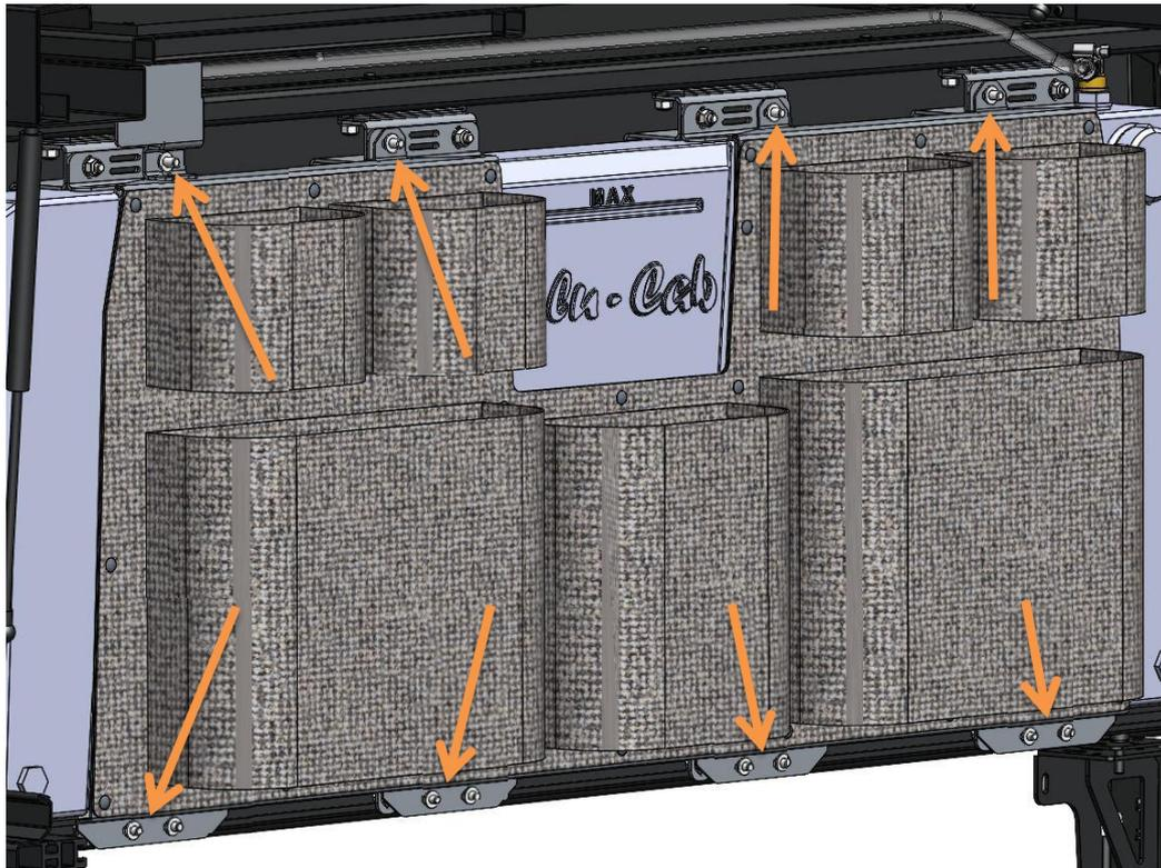
Place M8 Flat Washers over the shown Screw fasteners
