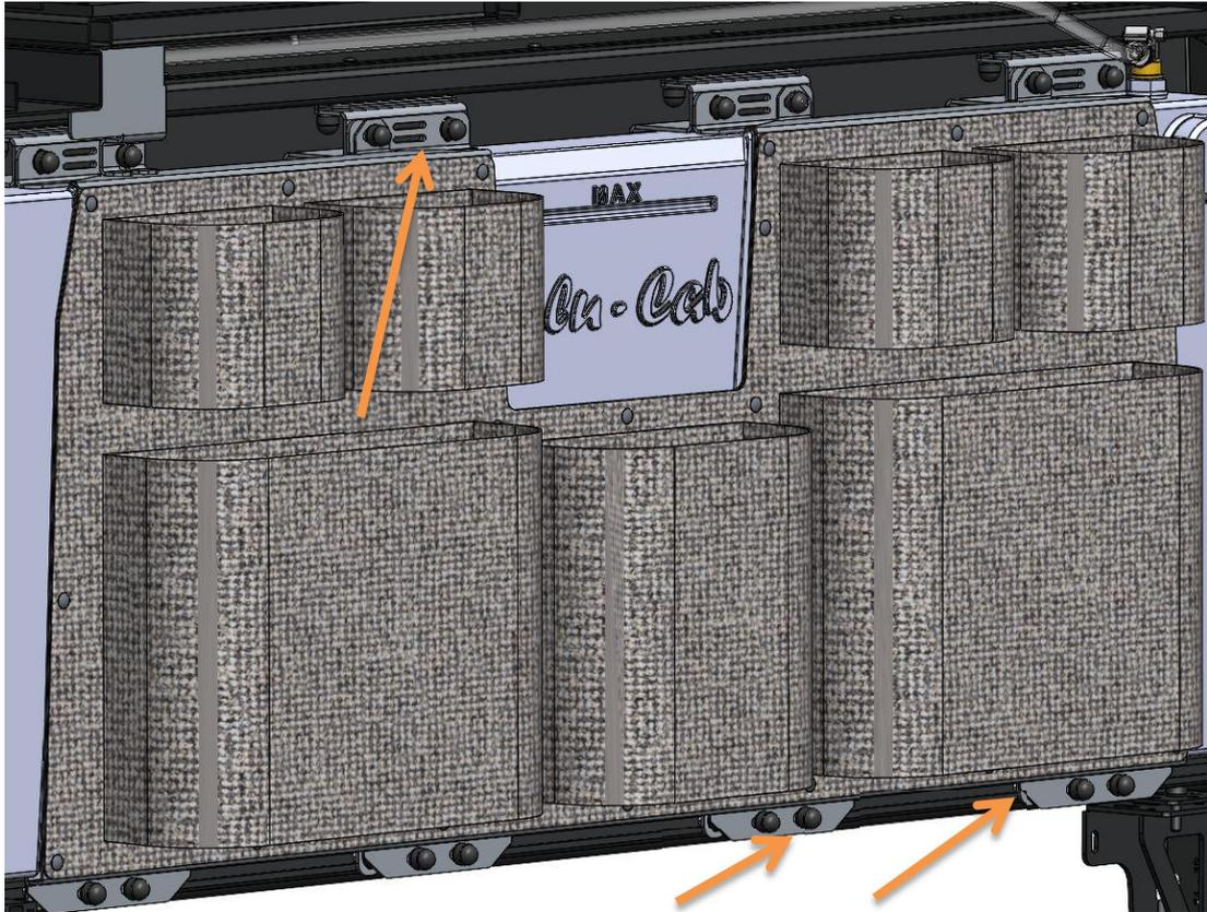
Place Plastic Nut Caps over all the exposed M8 Nuts and Screws
