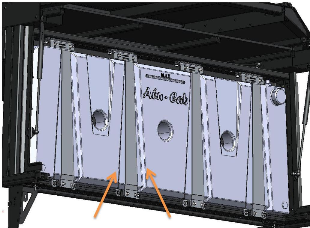
Place the Top Mounting Down Brackets over the Water Tank, between the Tank Ridges, as shown.
