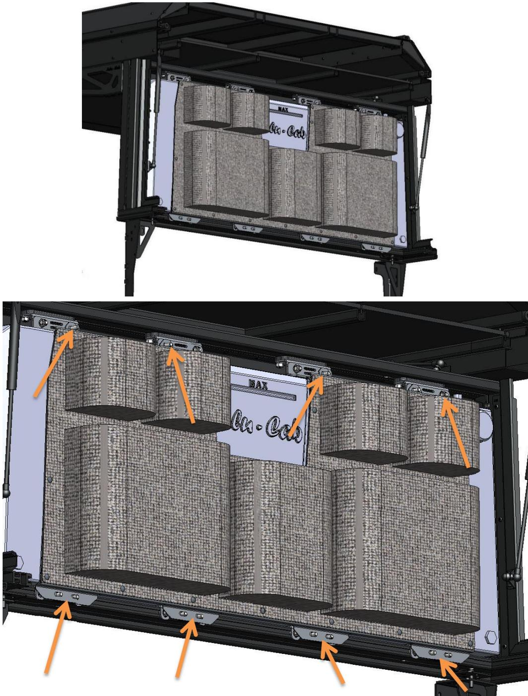
Place the Water Tank Cover Plate and Canvas Bag assembly over the corresponding Screw fasteners as shown
