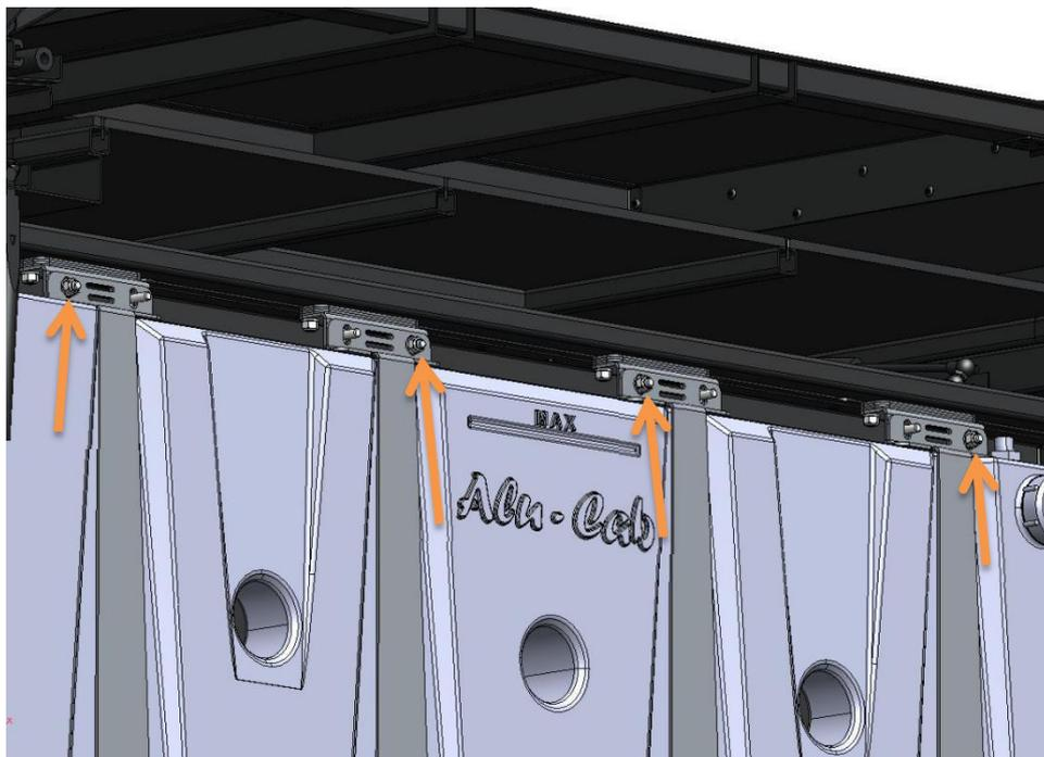
Secure the Top Mounting Down Brackets at the top using 4x M8 Nyloc Nuts
