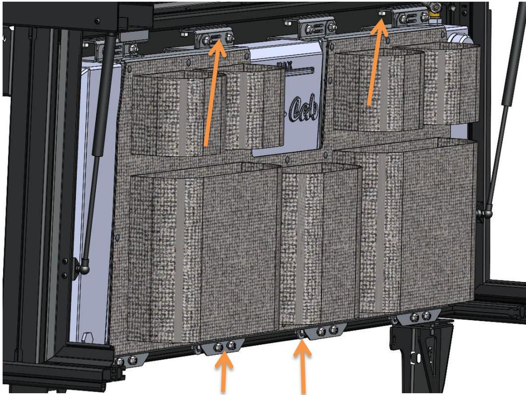
Fully tighten all Nyloc Nuts to secure the Water Tank in place
