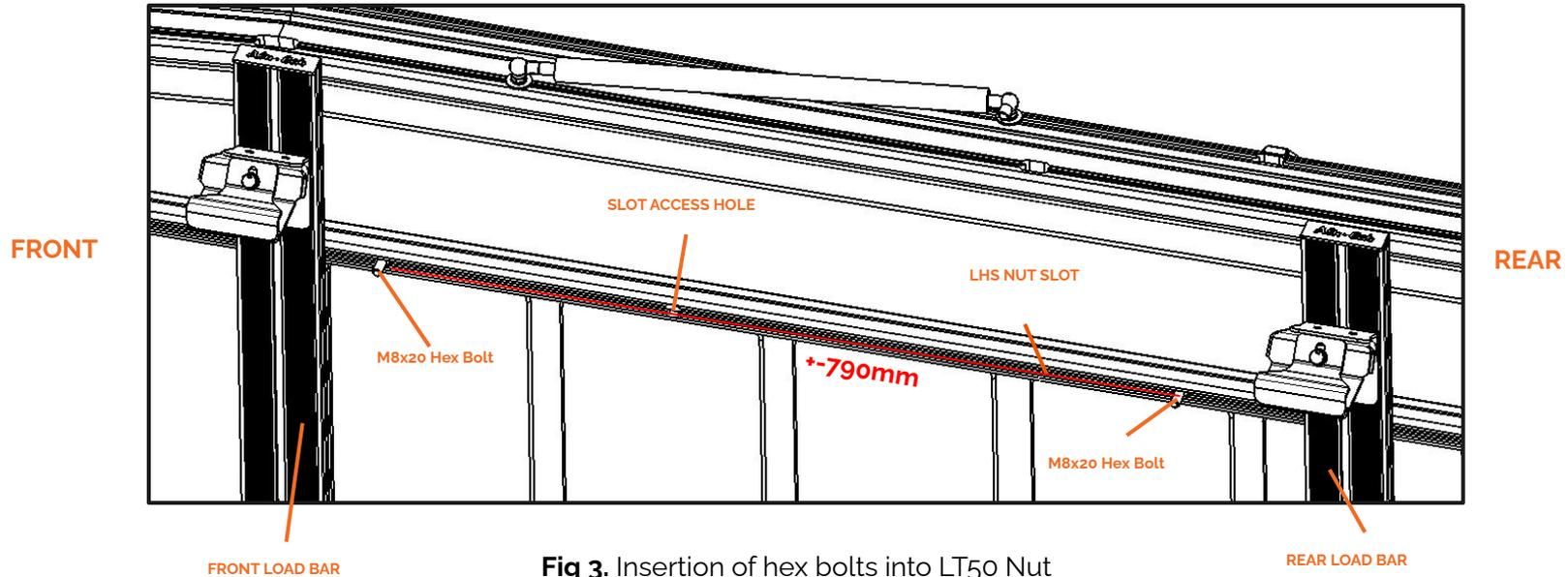
**Fig 3.** Insertion of hex bolts into LT50 Nut Slots
